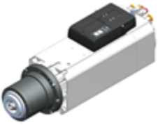
ES951 - Kw 25-S1/30-S6 - HSK E63 - liquid - long nose max speed 18.000rpm - rated speed 10.000rpm
