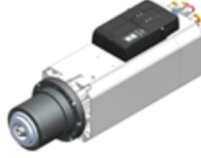
ES951 - Kw 25-S1/30-S6 - HSK F63 - liquid - long nose max speed 18.000rpm - rated speed 10.000rpm
